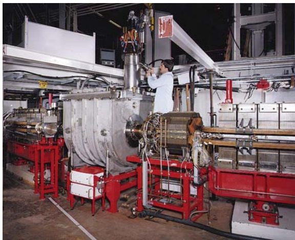
Fig. 3. Part of the machine lattice at SRS Daresbury. In the centre is the SRS superconducting wiggler 'wavelength shifter' at the time of its installation in 1981. Reproduced with the permission of Daresbury Laboratory.
